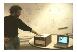
FIGURE 3.3.5 Retrieving information about a package by touching it. The box contains an electrostatically coupled RFID tag. Professor Gershenfeld is wearing a TouchTag reader in his shoe which reads the tag and outputs this information to the laptop. The laptop displays information about the box.
