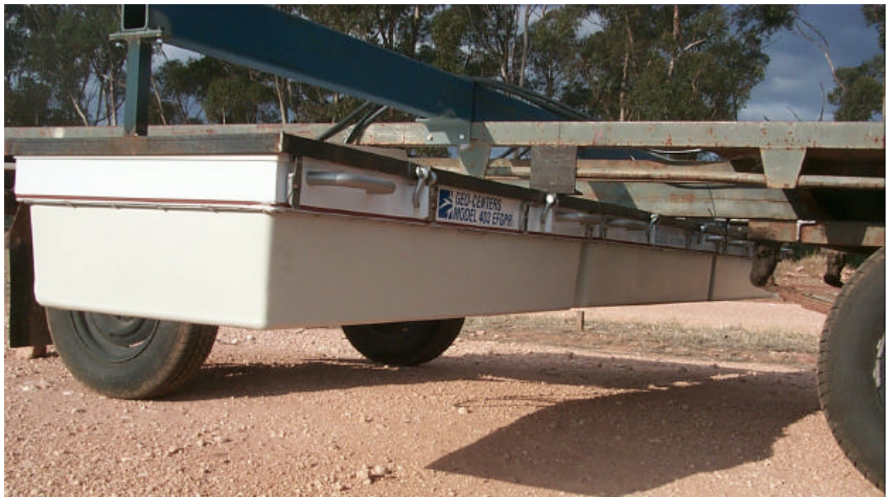
Figure 8. Three meter wide Model 403 EFGPR arrays in initial testing at Australia's Defense Science and Technology Organisation (DSTO).
