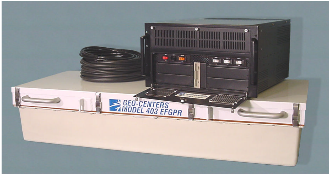
Figure 7. GEO-CENTERS Model 401 EFGPR with single array, cables and host electronics.
