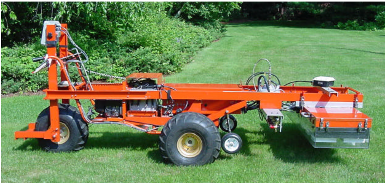
Figure 6: Model 401 EFGPR mounted on a self-propelled power wagon.
