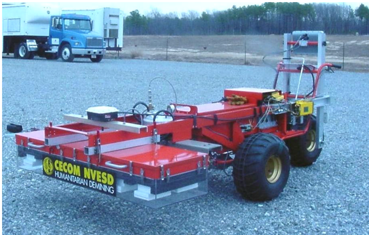
Figure 5. The Model 401 EFGPR on the 3 wheel man-portable platform developed for Fort Belvoir.
