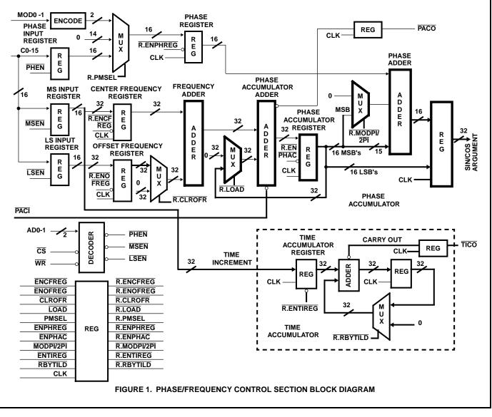
ment); the Time Accumulator supplies a pulse to mark the passage of a preprogrammed period of time.
