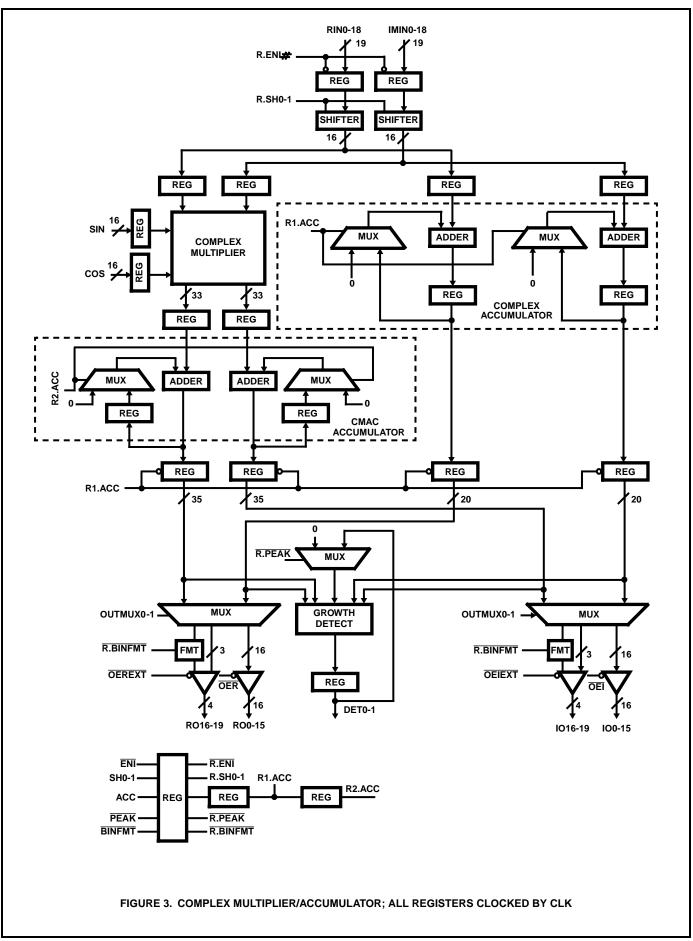
The Growth Detect circuitry outputs a two bit value that signifies the amount of growth on the data in the CMAC and Complex Accumulator. Its output, DET0-1, is encoded as shown in Table 5. If PEAK is low, the highest value of DET0-1 is latched in the Growth Detect Output Register.
