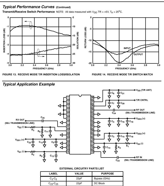
NOTE: All off-chip components are low cost surface mount components obtainable from multiple sources. (0.020in x 0.040in or 0.030in x 0.050in.)
