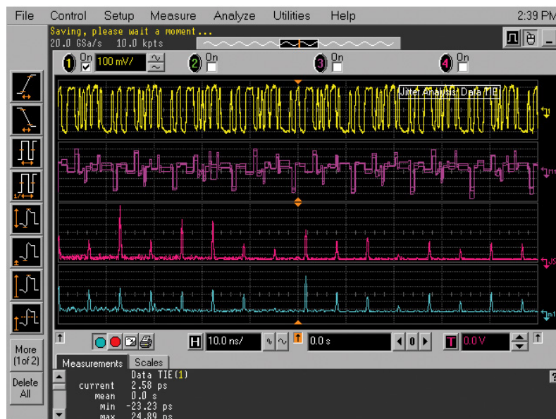
Figure 14: Detecting correlated Periodic Jitter (PJ)
