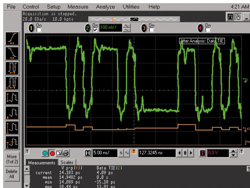
Figure 11: Testing for reflections at the transmitter side
