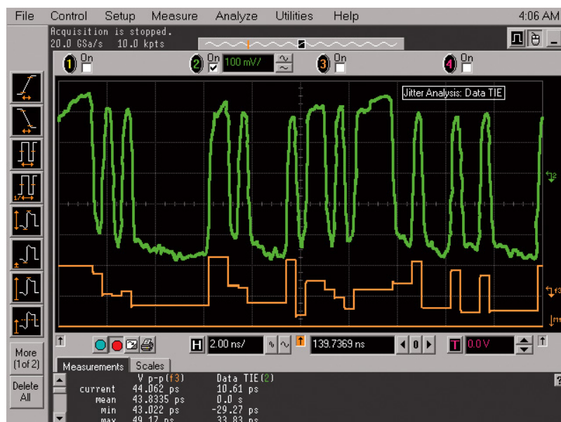
Figure 9: Isolating Inter-Symbol Interference (ISI)
