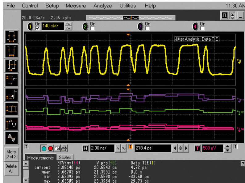
Figure 15: Measuring system Random Jitter (RJ)
