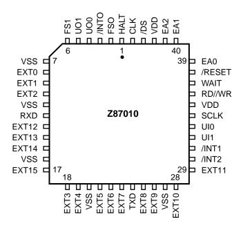
Figure 2. 44-Pin PLCC Pin Assignments
