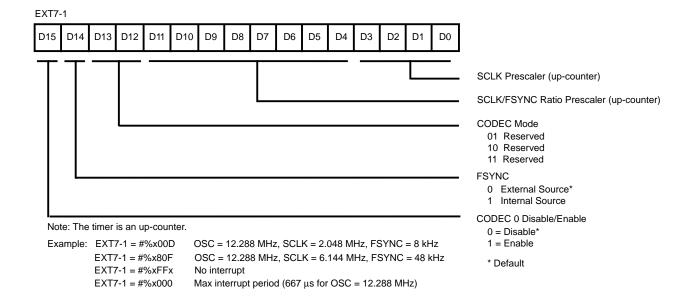
Figure 13. CODEC Interface Control Register
