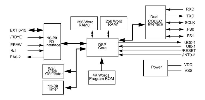
Figure 1. Z87010 Functional Block Diagram
