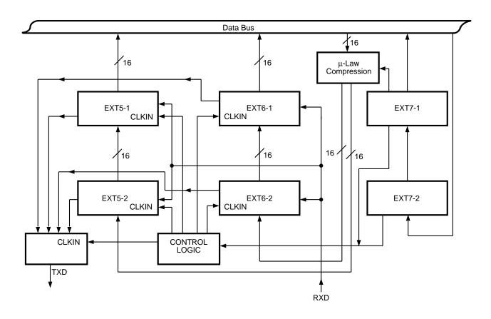
Figure 9. CODEC Interface Block Diagram
