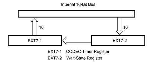
Figure 16. EXT7 Register Configuration
