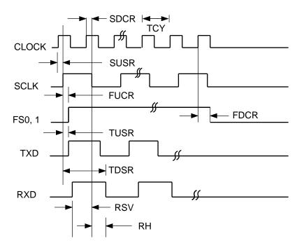
Figure 8. CODEC Interface Timing
