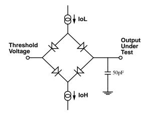
Figure 4. Test Load Diagram
