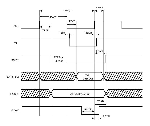
Figure 5. Write to External Device Timing
