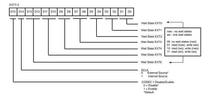
Figure 14. Wait/State/CODEC Interface Control Register
