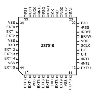
Figure 3. 44-Pin QFP Pin Assignments
