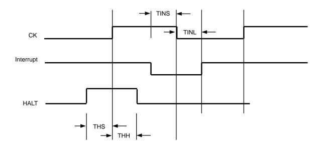
Figure 7. Interrupt/HALT Timing
