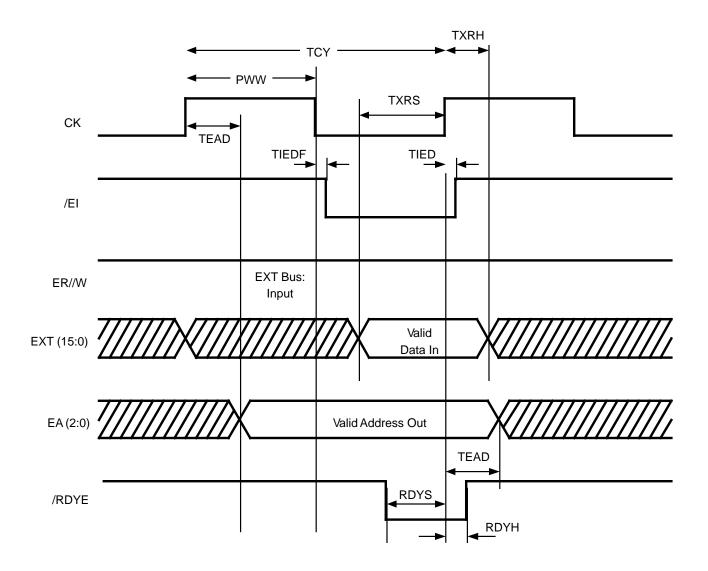
Figure 6. Read From External Device Timing
