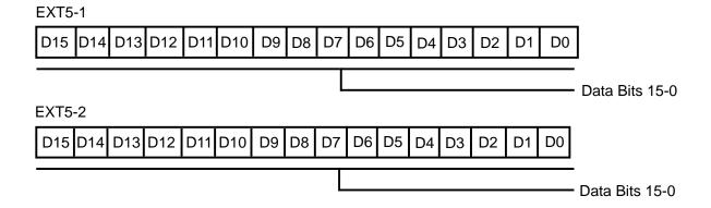
Figure 11. CODEC Interface Data Registers (Channel 0)
