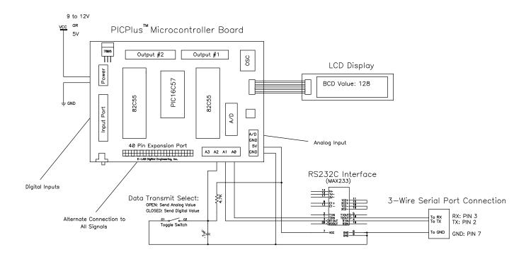
This application example illustrates the connection of the PICPlus<sup>™</sup> board to a PC via a RS232, 9600 baud serial connection. A Maxim 233 IC is used to make the physical connection.
