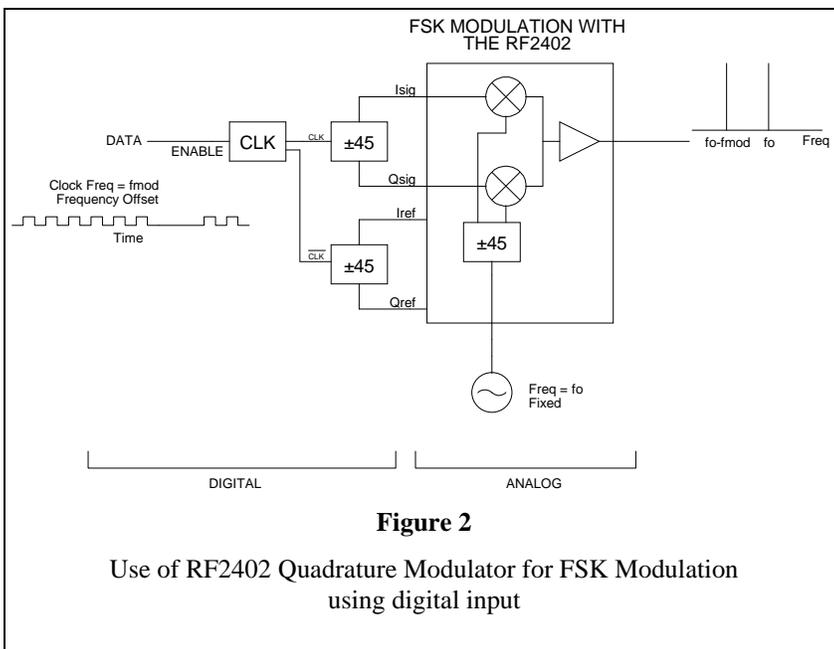
**OPERATING A QUADRATURE MODULATOR AS AN FSK MODULATOR**
